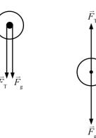
$$\begin{aligned} & \text{High} & \text{Low} \\ & F_{\text{c}} = F_{\text{T}} + F_{\text{g}} & F_{\text{c}} = F_{\text{T}} - F_{\text{g}} \\ & F_{\text{T}} = F_{\text{c}} - F_{\text{g}} & F_{\text{T}} = F_{\text{c}} + F_{\text{g}} \end{aligned}$$
